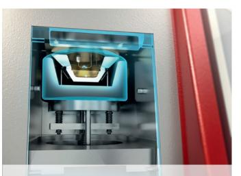
Ignition inside the continuously closed chamber formed by the sample cup and the oven plate
