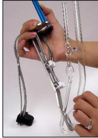
Figure 4. Inserting Base of Viscometer
