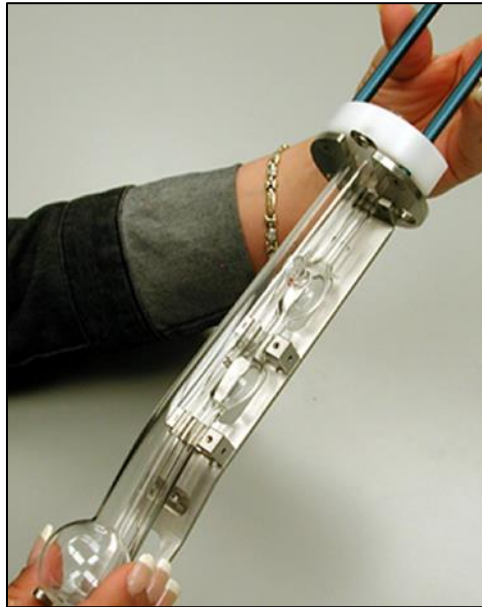
Figure 7. Viscometer Tube Completely Inserted in the Optical Sensor Assembly with Teflon® Ring. (Optical wires are not shown for illustrative purposes only.)
