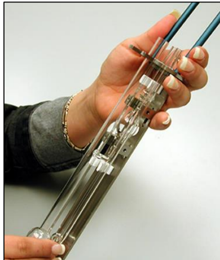
Figure 6. Viscometer Tube Completely Inserted in the Optical Sensor Assembly. (Optical wires are not shown for illustrative purposes only.)
