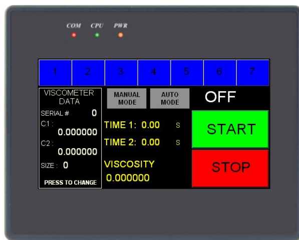
Figure 13. Control Panel (Main Screen)
